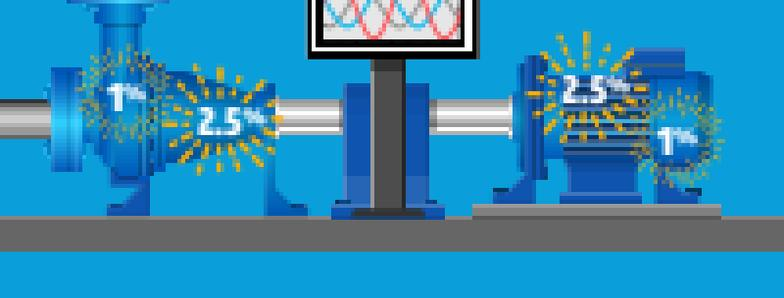
For a 100 hp motor operating 8,000 hours per year, a correction of the voltage unbalance from **2.5%** to **1%** will result in electricity savings of **9,500 kWh.**<sup>2</sup>
